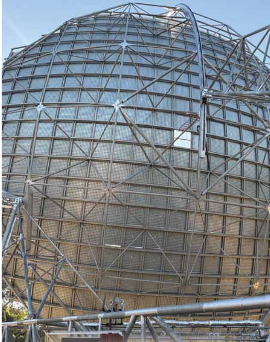
A giant solar concentrator installed at the Muni Seva Ashram, Vadodara, by RC Bombay Pier.
